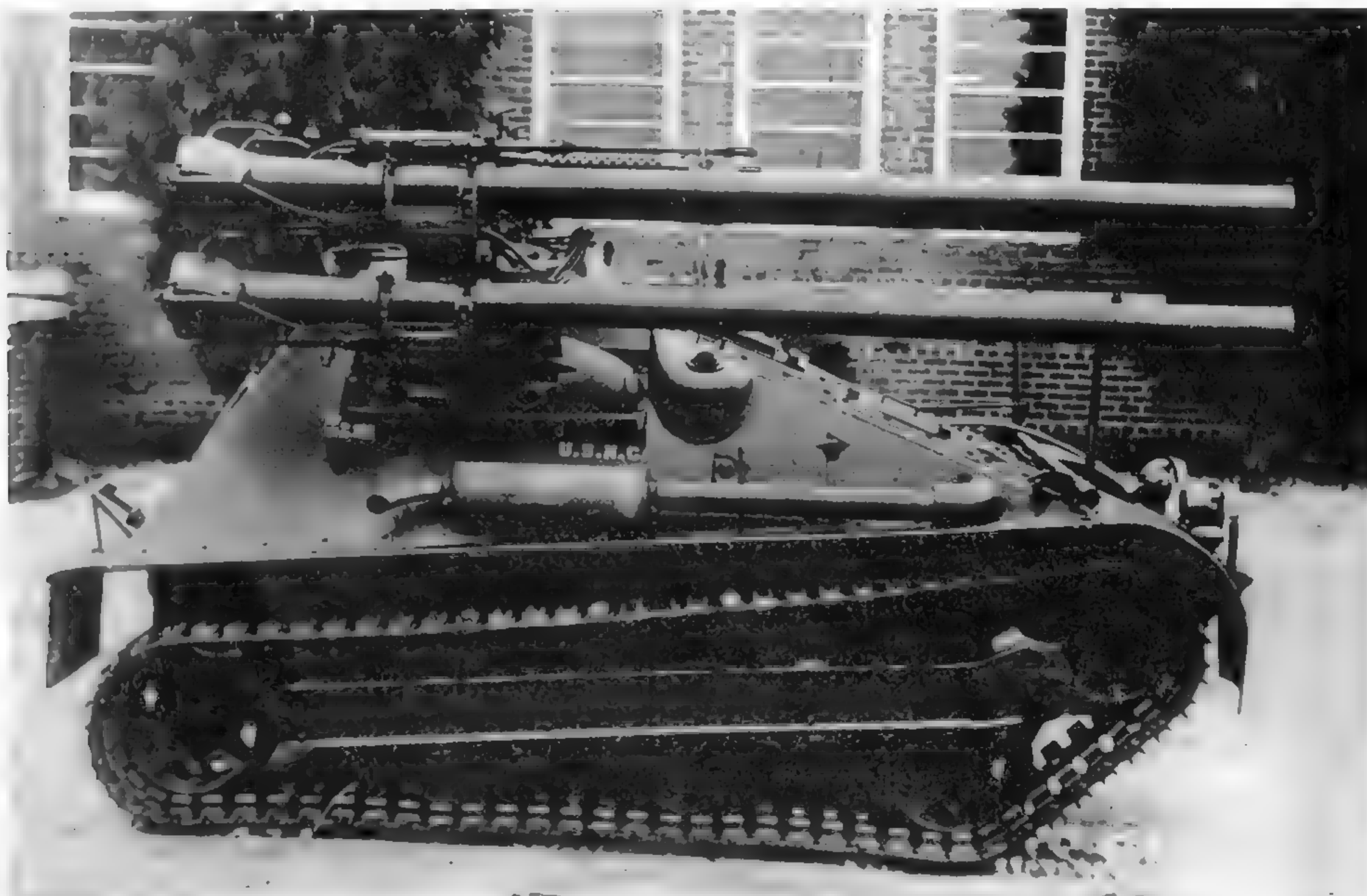
The upper outside 106mm recoilless rifle on each side of the Ontos (rifles 2 and 5) was designed to be quickly dismantled for ground use. These two tubes had M8C .50-caliber spotting rifles mounted on top of them. This type of spotting rifle was also mounted on top of tubes three and four. Barely visible in the center of the Ontos is an M1919A4 .30-caliber machine gun provided for self-defense. (Photo courtesy of the Patton Museum)
